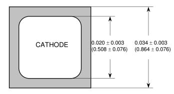
Bottom side metalization: AI - 25 kÅ minimum or Ti/Ni/Ag - 30 kÅ minimum. Top side metalization: AI - 25 kÅ minimum or Ti/Ni/Ag - 30 kÅ minimum. Bottom side is anode, top side is cathode.
